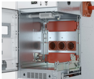
Independently operated and lockable shutters allow for safe cable or busbar testing while adjacent compartments remain live.
